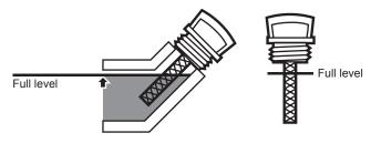
Add the appropriate type of oil until the oil level is at the full level. SAE 10W-30 oil is recommended for general use.
